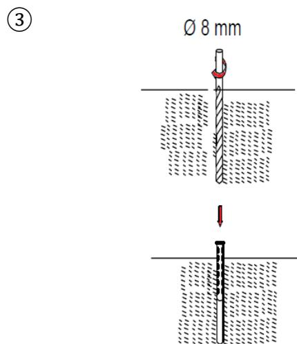
Drill 3 holes with drill bit ( $\phi$  8mm) on concrete surface, then insert anchors into holes.
