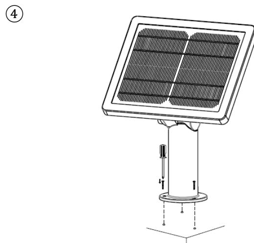
Install solar panel assembly on the surface with 3 screws.
