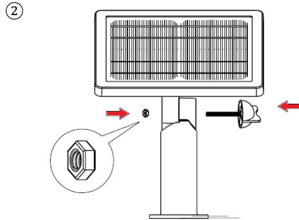
Fasten the parts together with butterfly wing screw and nut.
