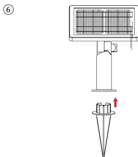
Alternatively, the solar panel could be installed on ground with using the spike.
